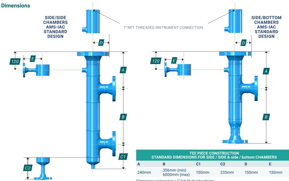
\*Dimensions are based on a 3" Sch 40 chamber design.
